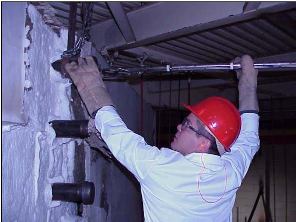
Fig. 12. Inserting particulate testing probe into breaching.
